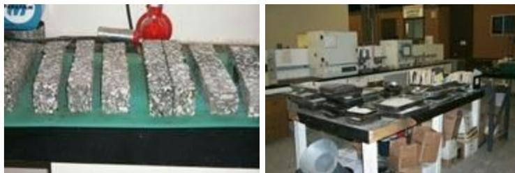
Different measuring techniques are used in the field than in the laboratory. In the field engineers use huge quantities of each rock size and weigh them on scales as large as a garage. In the laboratory, much smaller quantities of each material are needed and ordinary measuring utensils are used.
