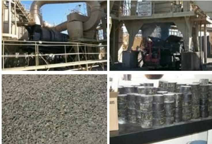
Paving materials, like asphalt, are manufactured in a plant. An asphalt plant has many parts. There are areas to store and weigh the construction materials, machinery to make the asphalt and a laboratory to test samples for strength and durability.
